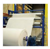
In many processes (coating and laminating, for example), the material speed affects the quality of the end product, making it desirable to maintain consistent web speed,
