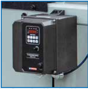
Variable Speed Core Drive for Best Cutting Speed
