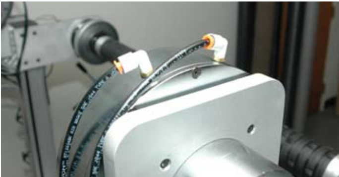
Air lines on a pneumatic chuck.
