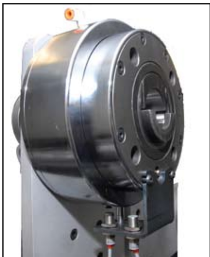
Pneumatic Safety Chuck with Proximity Sensors
