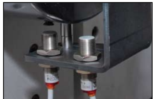
Open and Closed Proximity Sensors
