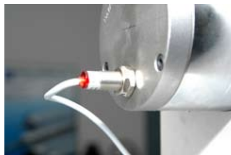
Rear sensor on a pneumatic safety chuck (idler side).
