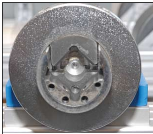
Safety Chuck without Radial Driver
